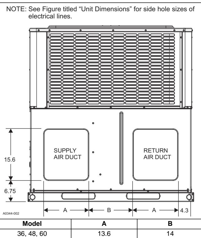
**UNIT TYPICAL DUCT APPLICATIONS**
