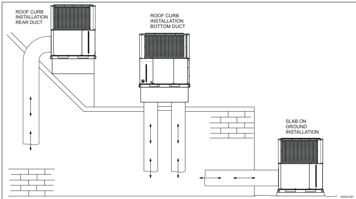
**UNIT TYPICAL SLAB ON GROUND INSTALLATION**
